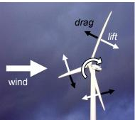
The blades of a modern wind turbine turn because of *lift*, the same force that makes it possible for an
