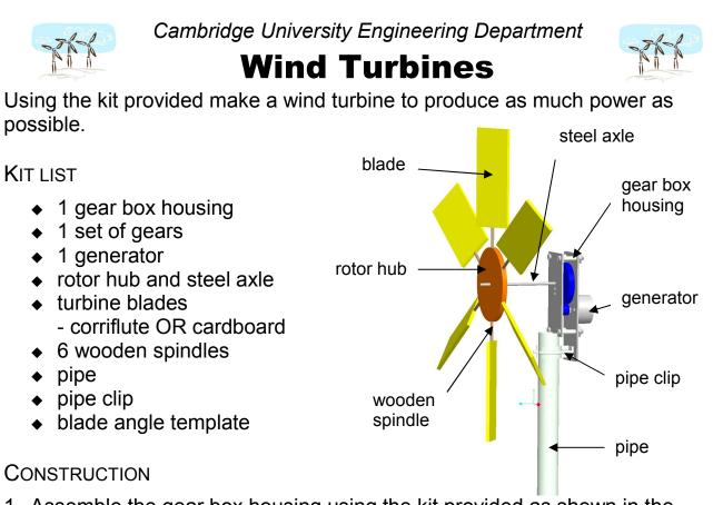
1. Assemble the gear box housing using the kit provided as shown in the exploded diagram. The smallest gear is connected directly to the generator.
