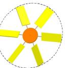
○ Top Tip: Remember that the wind from the fans we are using covers a limited area – if the blades are longer than this, the power will decrease. Larger blades are also heavier which increases *drag*. This means that the wind will have to be stronger to be able to start turning the turbine.
