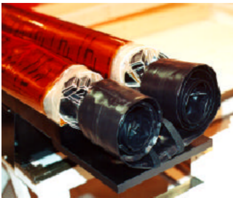
Figure 1.4: JPL's inflatable SAR frame. The antenna membrane and supports are stored rolled up (left).
