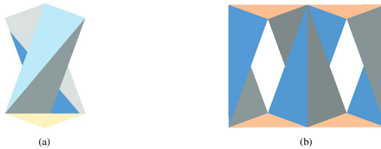
Fig. 13. The compact and deployed configuration of the network linked with scissor linkage
