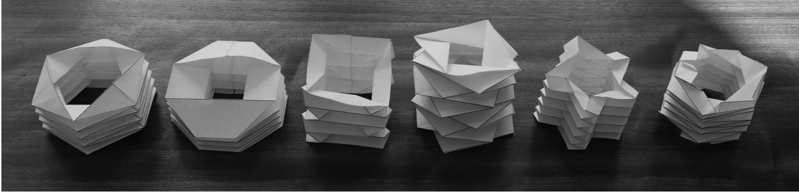
Fig. 3 Paper cylinders folded using fold patterns described in this section. From left to right: hexagonal Yoshimura pattern; tetragonal bellows fold; double-inversion bellows, with its derivative triangulated pattern; pentagonal Miura pattern; helically triangulated cylinder with hexagonal cross-section.
