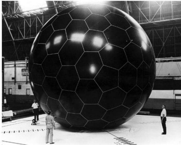
Fig. 19 The OV1-8 satellite with photolysable inflatable bladder embedded in a wire frame mesh (image credit: USAF).
