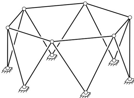
Figure 3: A ring structure with a finite mechanism.
