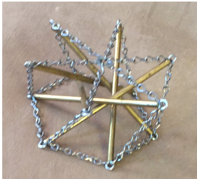
Figure 11.13: A super stable rotationally symmetric tensegrity with a star on the top and a regular hexagon on the bottom.
