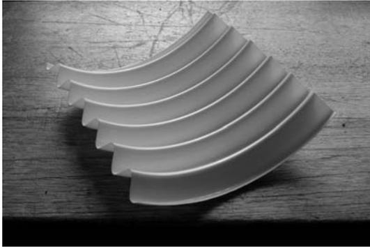
(a) The initial shape, unidirectionally curved along the corrugations.
