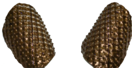
Figure 5: A doubly corrugated shell showing two twisted synclastic stable states.
