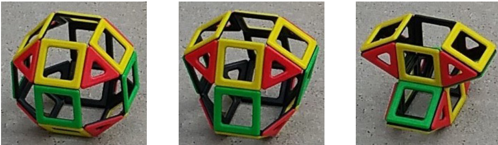
Figure 1: Physical models of W, R and B, constructed from Magnetic Polydron™ components. Rows (a), (b) and (c) correspond to W, R and B, respectively. Each row shows points on the path of the characteristic mechanism: initial high-symmetry configuration; the distortion mechanism, showing the halving of the symmetry group; the fully collapsed configuration after the pathway has passed through the multifurcation.
