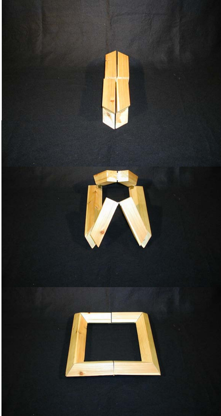
Figure 2.9: A simple model of the six-bar foldable frame.
