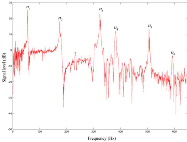
Fig.12(a): Resonance spectrum (0-650 Hz) of a 20 kN pre-stressed rod
