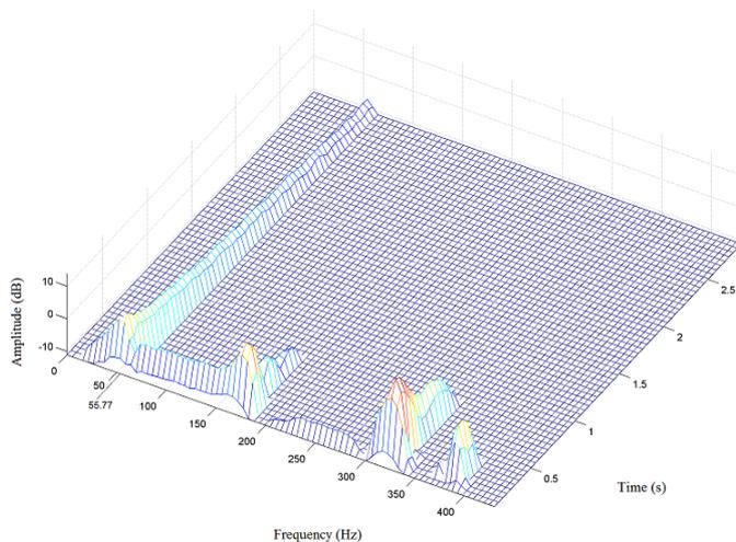
Fig.13: Sonogram surface plot showing the natural modes of vibration in a range 0-400 Hz.
