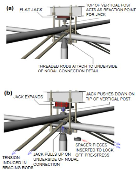
Fig. 6: Jacking method 1. (a) The jack is set up on node of the vertical post, (b) the jack pushes the tip of the extending rod and a spacer creates the extension.
