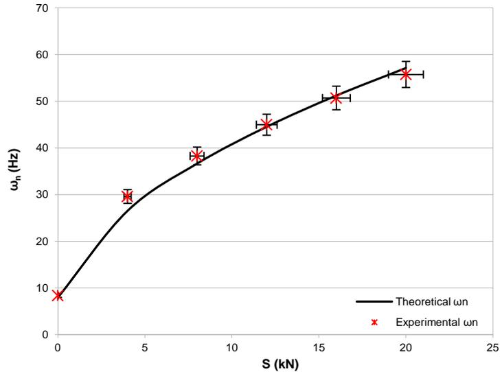
Fig.15: Experimental  $\omega_n$  with 5% error bars fitted on the theoretical curve produced from eq. (1).
