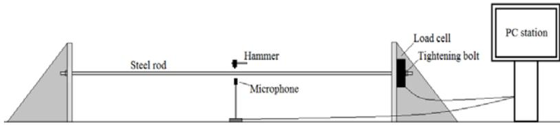
Fig.11: Diagram of the experimental setup used to obtain the acoustic resonance spectrum of the cylindrical tension rod when stretched to a certain tensile load.
