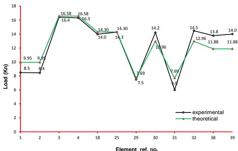
Fig. 8: Theoretical vs Experimental tensile loads carried by the diagonal pairs after a 2mm extension using pre-stressing technique (b).
