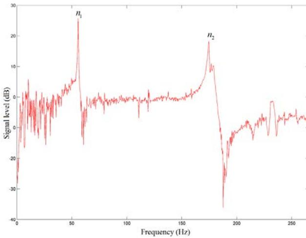
Fig.12 (b): Resonance spectrum (0-250 Hz) of a 20 kN pre-stressed rod.
