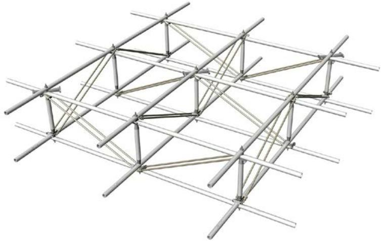
Fig. 3: The 2×2 double layer tensegrity grid with SS=1 and IM=4.
