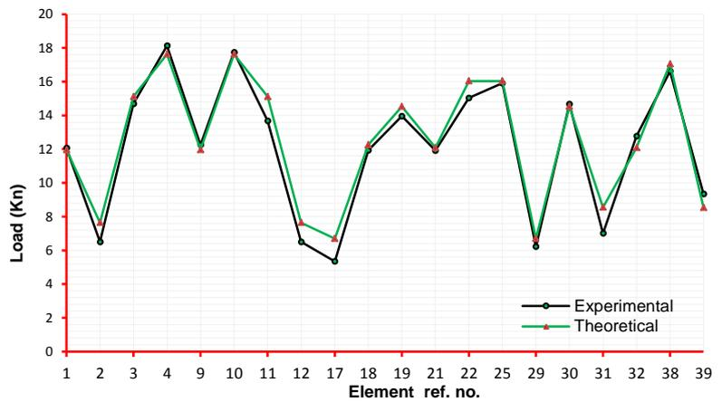
Fig. 10: Theoretical vs Experimental compressive loads carried by the vertical elements after a 2mm extension and a 12.7 kN applied load using pre-stressing technique (b).
