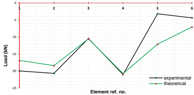
Fig. 9: Theoretical vs Experimental compressive loads carried by the vertical elements after a 2mm extension using pre-stressing technique (b).
