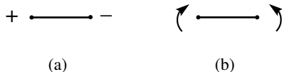
Figure 2. Representation of (a) the single state of self-stress, and (b) the single mechanism, of the double banana. Each vertex represents a banana: in (a), the + or – represents an overall state of tension, or compression; in (b), the arrow represents rotation of the banana around the shared implied edge.
