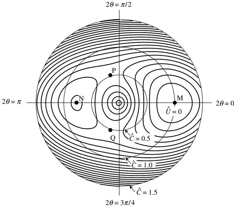
Figure 8. Polar plot of non-dimensional energy  $\hat{U}$  versus  $\hat{C}$  and  $\theta$  for the antisymmetric composite shell example. Contours are plotted at  $\hat{U} = 0.05, 0.1, 0.15, \dots$ . The four equilibrium points are labelled M, N, P and Q.
