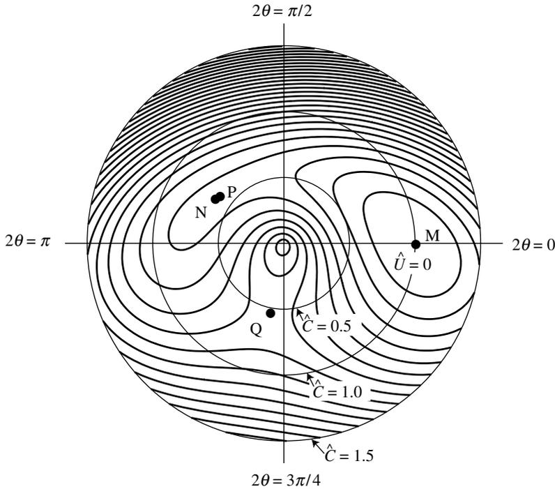
Figure 9. Polar plot of non-dimensional energy  $\hat{U}$  versus  $\hat{C}$  and  $\theta$  for the symmetric composite shell example. Contours are plotted at  $\hat{U} = 0.05, 0.1, 0.15, \dots$ . The four equilibrium points are labelled M, N, P and Q.
