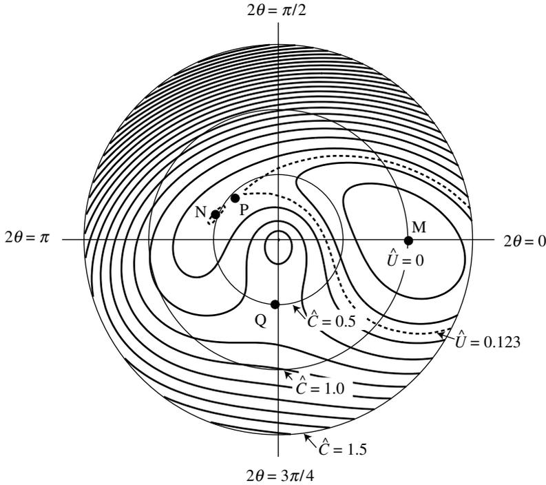
Figure 10. Polar plot of non-dimensional energy  $\hat{U}$  versus  $\hat{C}$  and  $\theta$  for the  $40^\circ$  symmetric composite shell example. Contours are plotted at  $\hat{U} = 0.05, 0.1, 0.15, \dots$ . The four equilibrium points are labelled M, N, P and Q. The additional contour  $\hat{U} = 0.123$  has been plotted as a dashed line to show more clearly the nature of the equilibria at N and P.
