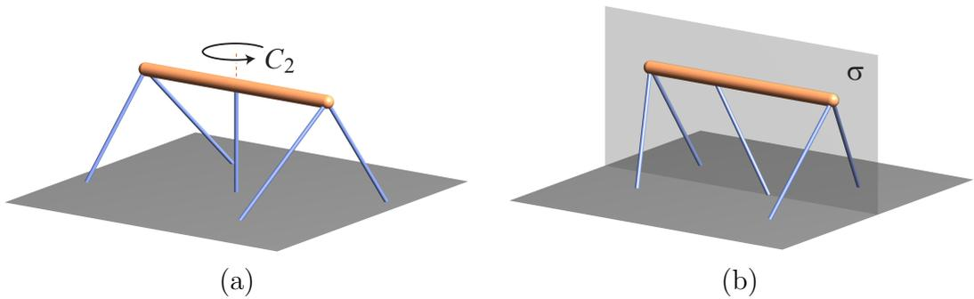
Figure 8: Two symmetric configurations of the linear pentapod, one with half-turn symmetry (a) and one with reflection symmetry (b).
