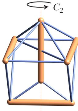
Figure 3: A rod-bar framework with an isostatic scalar count that has an infinitesimal motion and a state of self-stress, both detected by calculations of the symmetry-extended mobility count. In this and subsequent figures, rods are schematically depicted as ‘wooden’, and bars as ‘metallic’.
