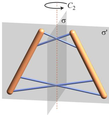
Figure 9: A rod-bar framework with  $C_{2v}$  symmetry. As it lies within the mirror plane corresponding to  $\sigma'$ , it is not isostatic.
