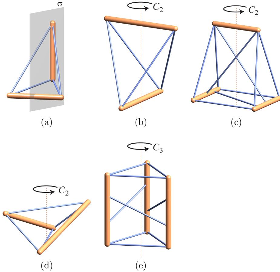
Figure 5: Isostatic symmetric rod-bar frameworks, with their point-group symmetries ((a)  $\mathcal{C}_s$ ; (b),(c),(d)  $\mathcal{C}_2$ ; (e)  $\mathcal{C}_3$ ), exemplifying the various structural counting rules derived in the text.
