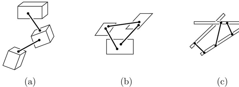
Figure 1: Frameworks in 3-space: (a) A *body-bar* framework, (b) a *panel-bar* framework, and (c) a *rod-bar* framework. Dumbbell symbols indicate a bar and its two points of attachment.
