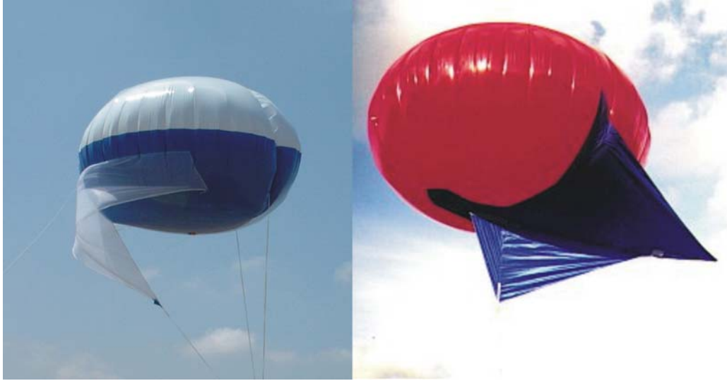
Figure 2.3: Examples of variable lift aerostats. The balloon on the left is the Skydoc ® from FLOATOGRAPH[37] and the one on the right is the Helikite ® from ALLSOPP[38]
