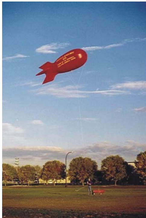
Figure 2.2: Example of streamlined aerostat. The picture shows a TIF-460 ® aerostat from Aerostar[36].
