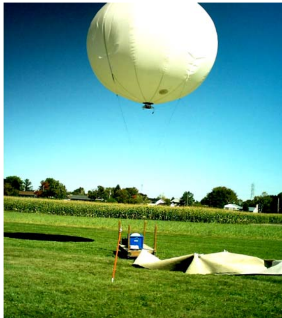
Figure 2.1: Picture of the physical platform. The black spot at the bottom of the balloon is the instrument platform.
