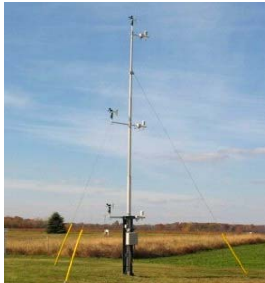
Figure 2.10: Picture of the wind tower with the Young wind sensors at 3, 5 and 10 m.
