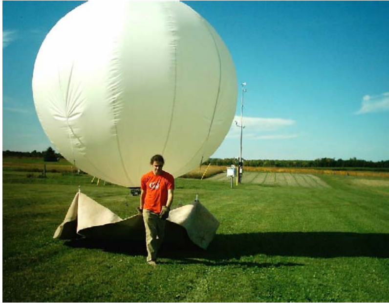
Figure 2.16: The ground handling of the balloon was performed by one person. A soft carpet was used to keep the balloon close to the ground
